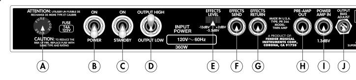
If a fuse blows, it should be replaced only with a fuse in accordance with the listing at the fuse holder. If the amplifier repeatedly blows fuses, it should be checked out by a qualified technician. UNDER NO CIRCUMSTANCES should a fuse of a different type or higher rating, or a fuse bypass be used, as this could damage the equipment and present a serious safety hazard.
