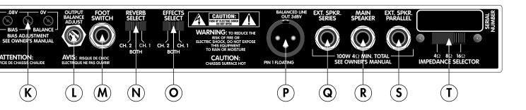
L. OUTPUT BALANCE ADJUST — Used in conjunction with the BIAS TEST POINTS (item K) to set the balance between the push/pull tube sections of the power amp. See output Tube Bias Adjustment Instructions below.
